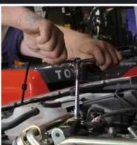
SIDCHROME Pico tool sets are a 1/4" drive multi-service socket and screwdriving tool sets ideal for all-round use. Each set features a highly versatile and ultra-compact rotating ratchet with 180-degree flexible head, which locks in all positions and is suitable for confined workspaces. All tool components come safely secured in a compact heavy-duty blow-mould storage case which is easy to carry and can be taken with you anywhere.
